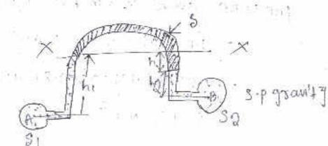
Let an inverted u-tube manametert connected to the 4-wo prints A and B let pressure at A is mure than pressurie at B consideri.
